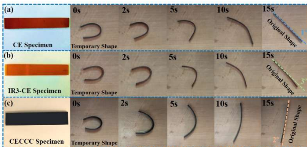
Figure 10. The shape recovery process of U-shape specimens at 190 °C.
