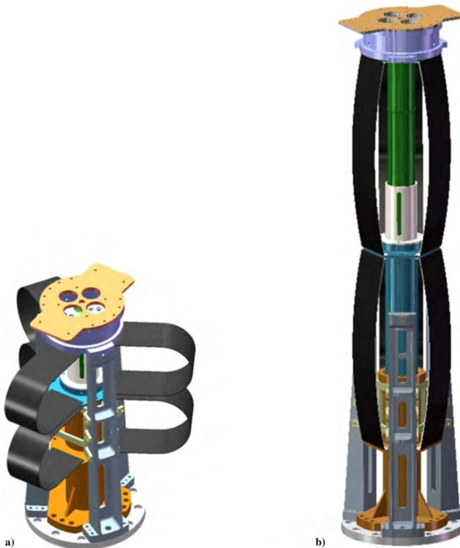
Fig. 2 Structural design of the SDT in a folded shape (a) and in a deployed shape (b).
