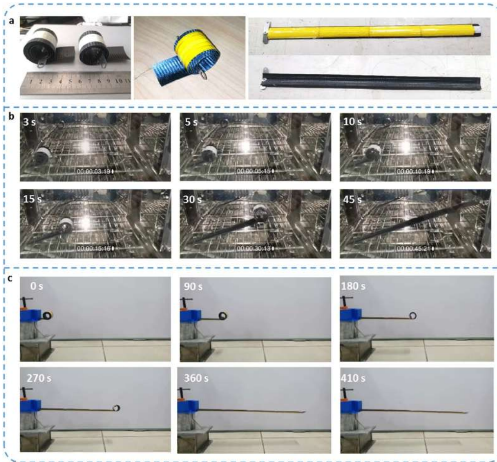
Figure 7. Deploying tests of the Bi-SMPC booms. (a) Folded state without heating circuit, folded state with the heating circuit, and deployed state of the Bi-SMPC booms, respectively; (b) deploying test of the Bi-SMPC boom in an oven; (c) deploying test of the Bi-SMPC boom driven by the heating layer at a voltage of 20 V.
